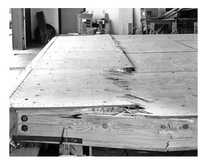
Figure 13-2 Plywood structural diaphragm testing. (Courtesy APA—The Engineered Wood Association)
